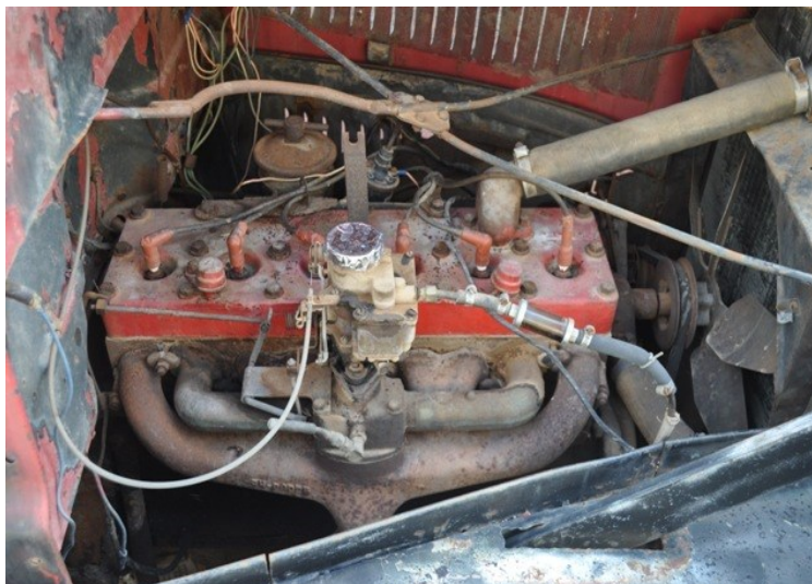
International 233 Green Diamond Motor as used in the USMC 1 ton M-2-4 Trucks 1943-1945
