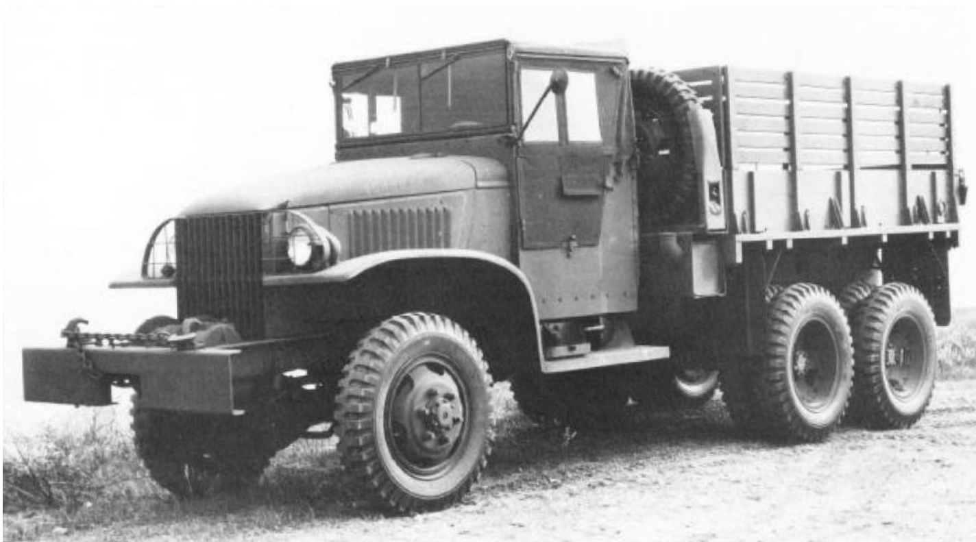
1944 GMC CCKW Short Wheel Base. This is a late model open cab with a wood bed. U.S. Army
