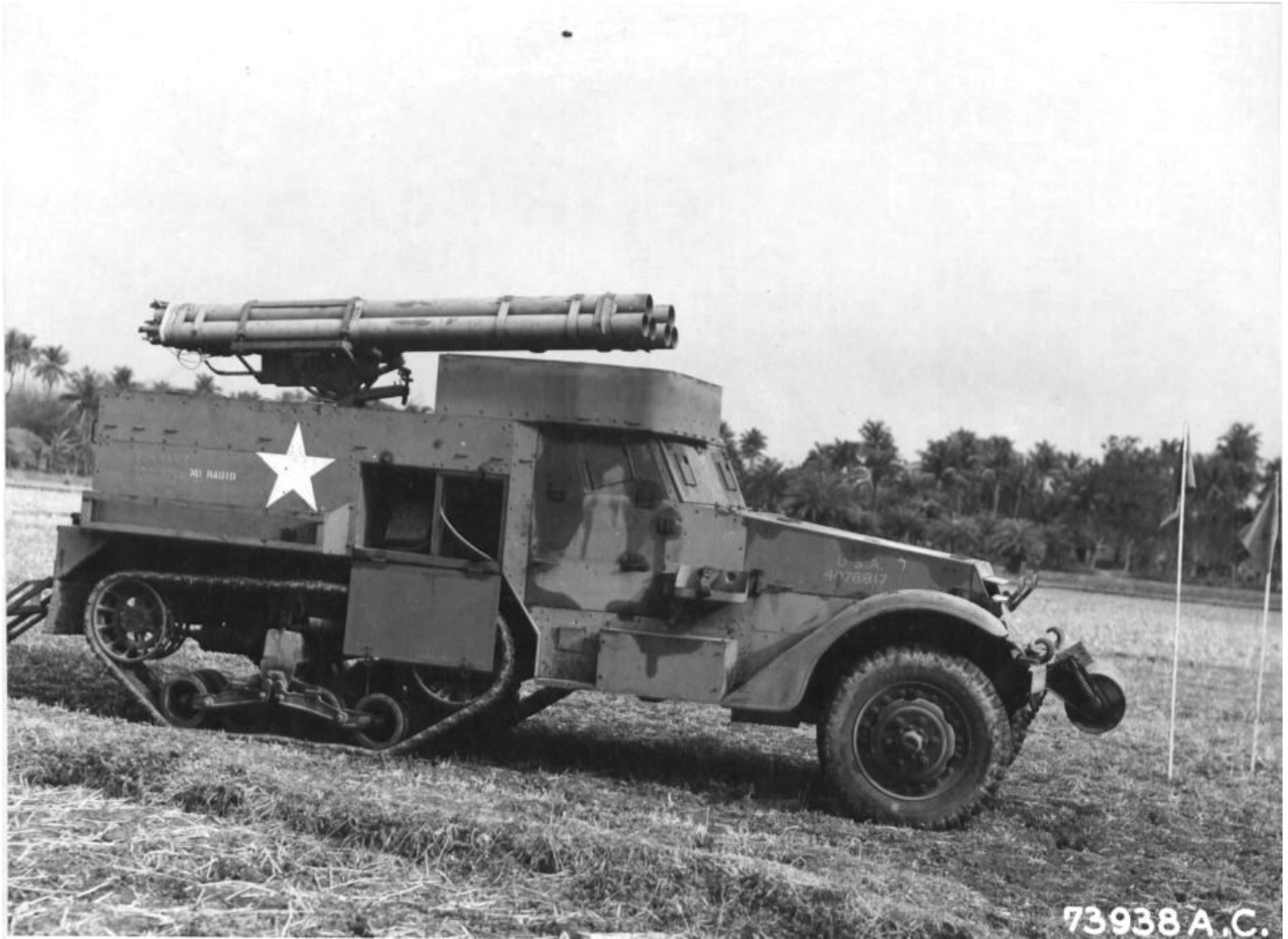
M3 Half-Track mounted with two 3-tube rocket launchers at the Bengal Air Depot near Calcutta (now Kolkata), India, 1942-45. U.S. Army
