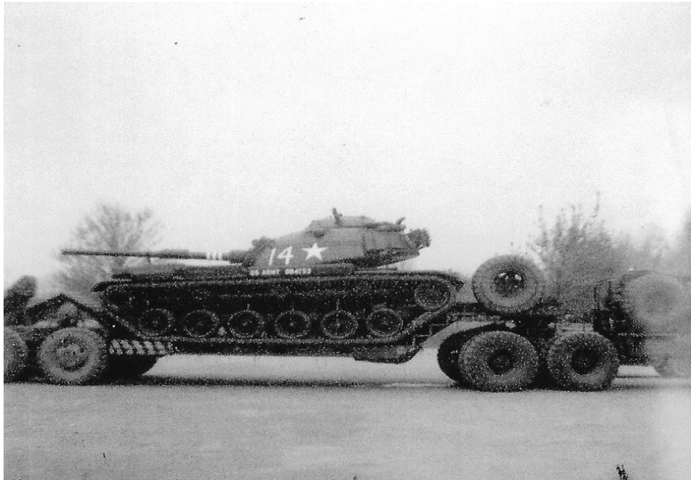
The 10 ton M123/M125s built in the 1950s had a LeRoi T-H844 a 844 cu in overhead valve V8 gasoline engine. M123A1s built in the 1960s had a Cummins V8-300, a 785 cu in V 8 diesel engine. This engine was also retrofitted into M123s to make M123E2s. Mack M123/125's drive train used much from the WW2 Mack NO. A very unique prime mover. Pictures from Carl Poerschke
