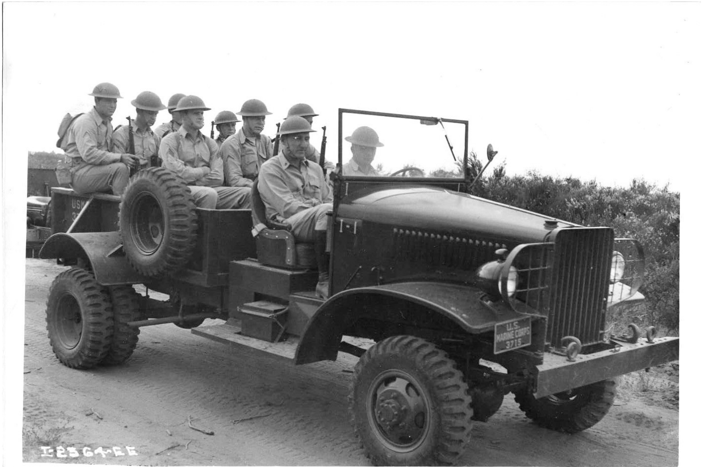
I-2364-EE--International Model M-1-4 4-wheel-drive truck, U. S. Marine Corps, loaded with marines on way to artillery range. Noncommissioned officer seated next to driver holds Marine Corps rating of gunner. Letter and number on cowl indicate truck belongs to "I" Battery, First Section. 2 1/4 x 3 1/4 negative. Houston.
