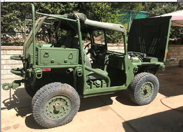
The “compact” PM 105: with roll bar and storage/tool boxes. Paul Baptist, NZMVC
